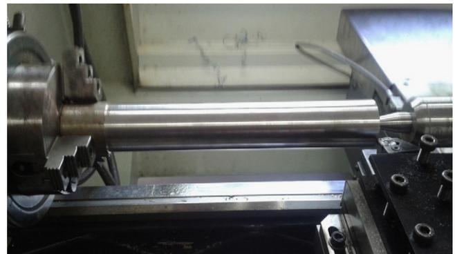
Fig. 2. AISI 12L14 steel machined on a CNC lathe with a 5.5 kW spindle motor with conventional roller bearings.
