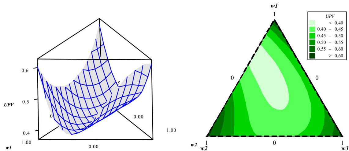
Fig. 9. UPV response surface and contour plot.
