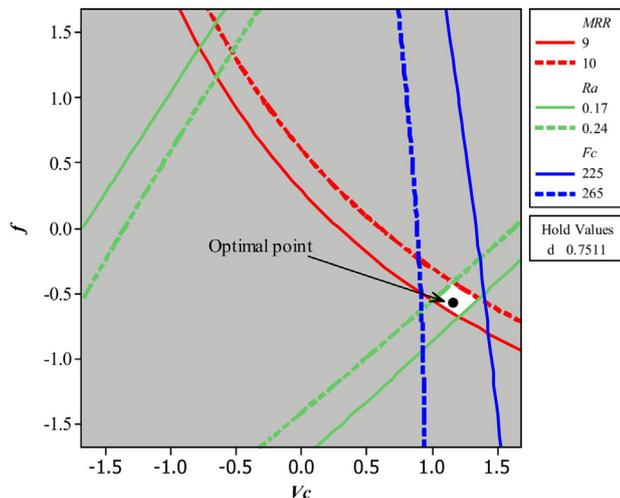
Fig. 11. Point of optimization for *MRR*, *Ra*, and *Fc*.
