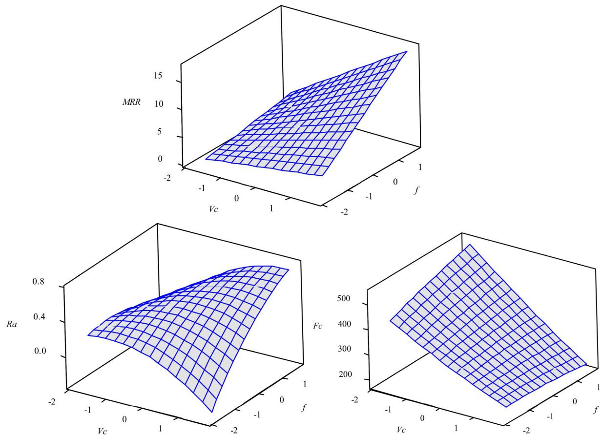
**Fig. 5.** Response surface for MRR, Ra and Fc (hold value:  $d = 0$ ).
