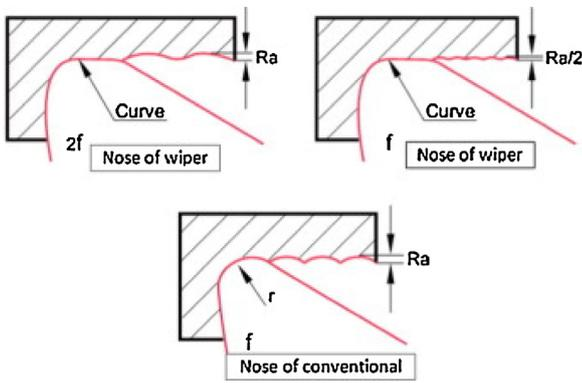
Fig. 1. Surface generation using wiper and conventional inserts [18].
