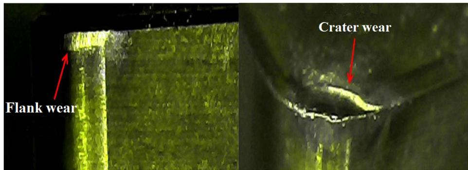
Fig. 2. SEM images of the flank and crater wear of cutting tool.
