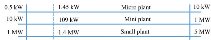
Fig. 3. Nominal power limits for each plant classification.
