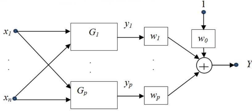
**Fig. 1** Typical RBF neural network structure.
